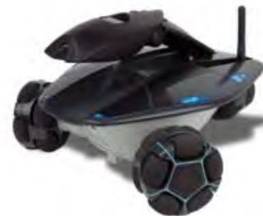
↑ The Rovio robotic webcam is wirelessly connected to the Internet. It roams around the home providing an audio and video link to keep an eye on family or pets when you're out.
